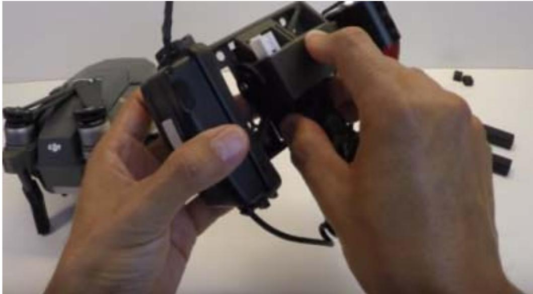
Observe the correct orientation of the Release & Drop PLUS Device and insert it into the SearchLight mounting plate as shown. The Release & Drop PLUS Device should tightly fit into the existing holes and slots of the SearchLight mounting plate.
