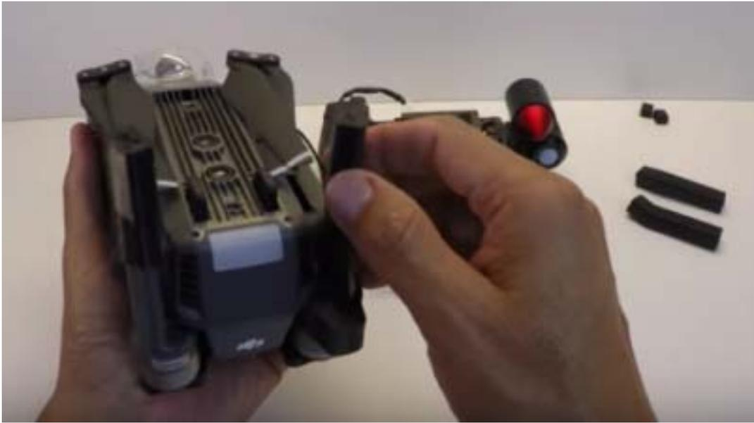
Remove the original landing gear feet that came with the Release & Drop PLUS Device
