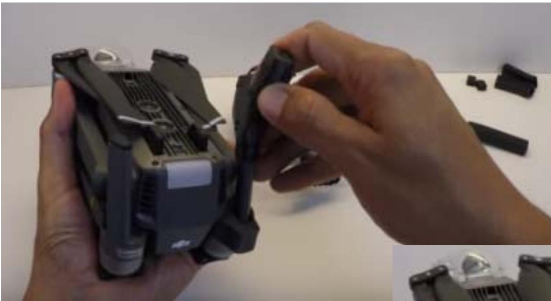
Install the extended landing gear feet (provided)
