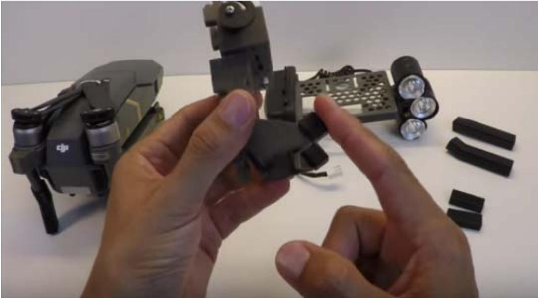
Remove the original landing gear feet
