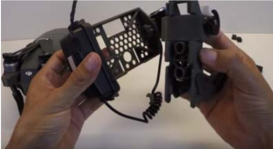
Correctly orient the Release & Drop PLUS Device with the SearchLight mounting plate as shown
