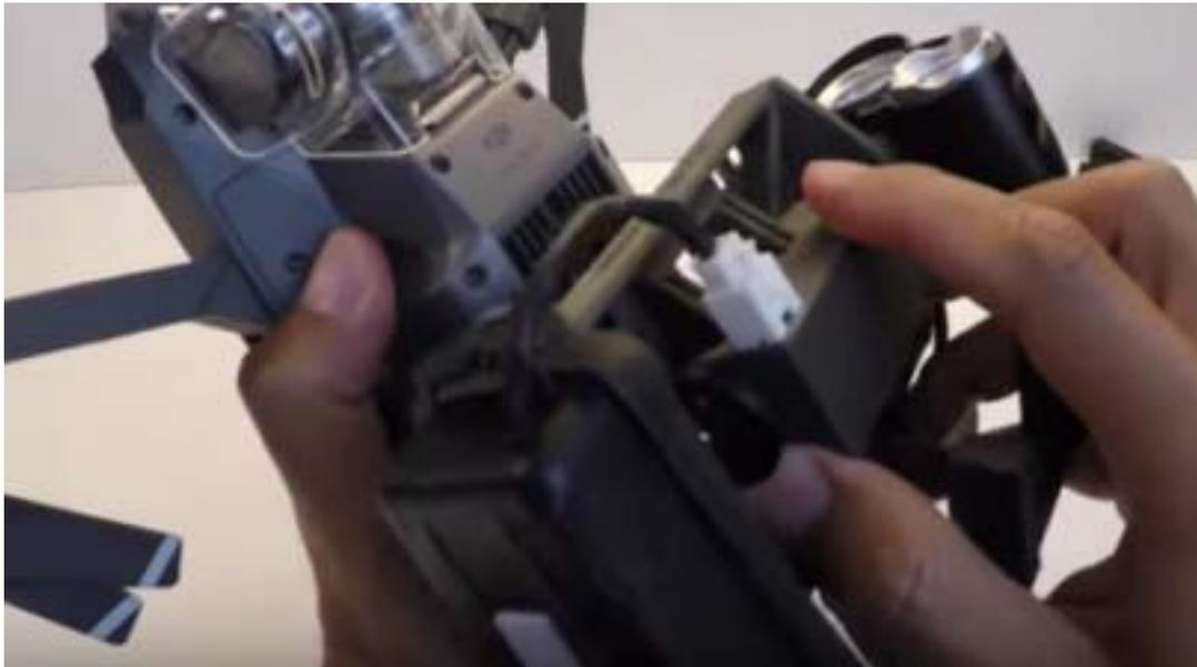
Slide the complete assembly (Release & Drop PLUS Device with the SearchLight) into the front slots of the Mavic's heatsink.
