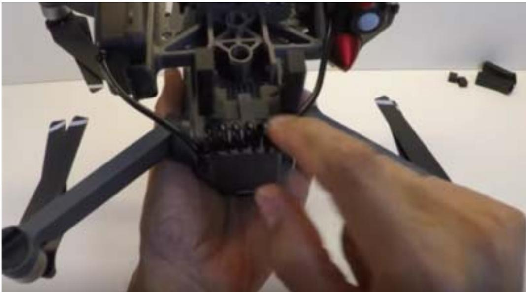
Lock down the coiled cable holder into the Release & Drop PLUS Device rear rotating bracket
