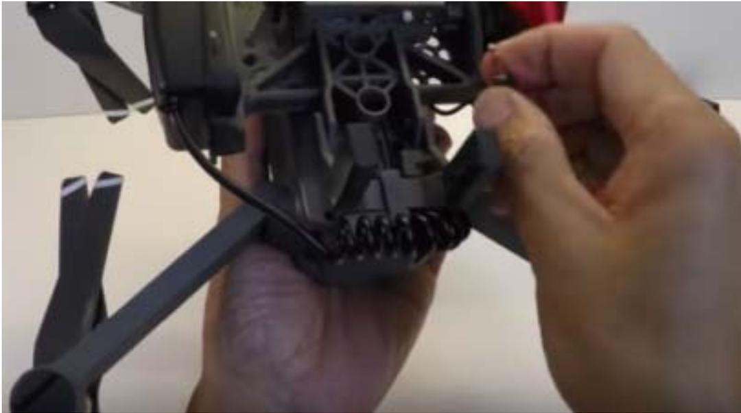
Route the Light Sensor cable under the SearchLight mounting plate and orient the cable plug towards its jack located on the Release & Drop PLUS Device.
