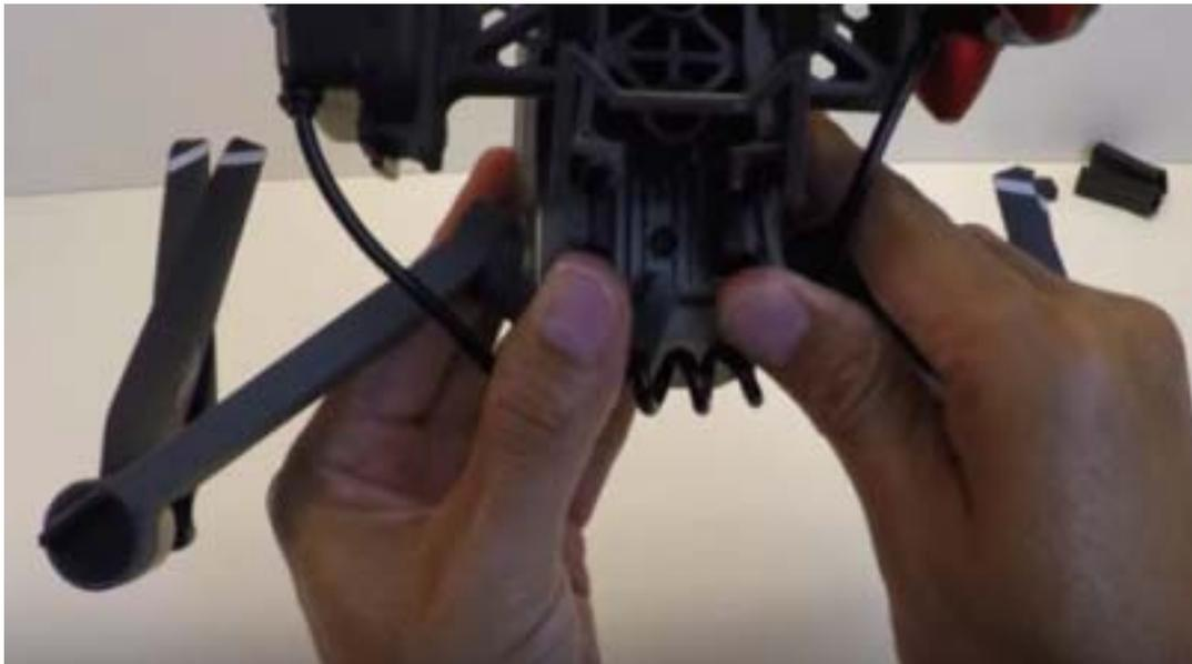
Spread the rear sides of the Release & Drop PLUS Device with your fingers and insert them into both holes of the Mavic's landing gear.
