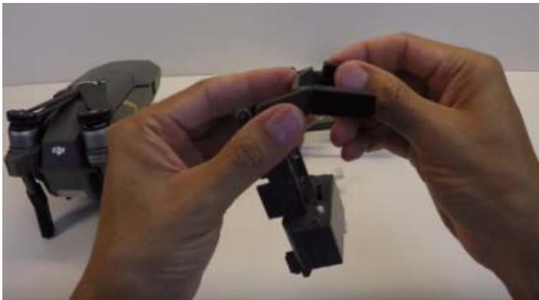
Install the extended landing gear feet (provided)
