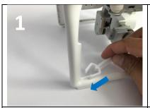
Slide the alignment pin bracket from the drone's inner side on both rear landing gear
