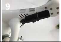
The LED Sensor should fully cover the drone's lens
