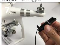
The LED Sensors is installed under the front right electric motor
