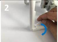
Turn the alignment pin bracket towards the bottom side of the landing gear until it locks
