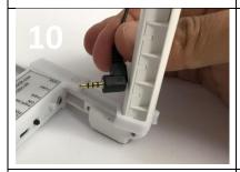
Fully insert the plug of the LED Sensor cable into the 'SENS' port on the Drone Sky Hook Arrow
