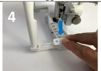
Align the Drone Sky Hook Arrow's hole with the alignment pin and press down on the Arrow until it locks to the landing gear
