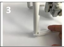
Verify that the alignment pin bracket is in-line with the bottom side of the landing gear
