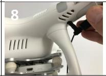
Slide the rubber band over the motor and insert the pin to the hole in the drone's arm
